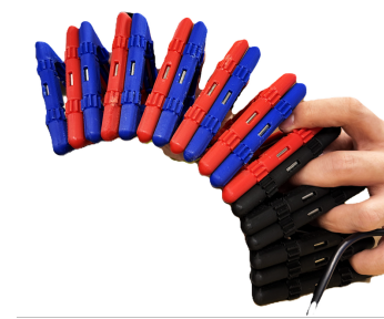
Fig. 8: Flexible bending enabled by simple stacking.
